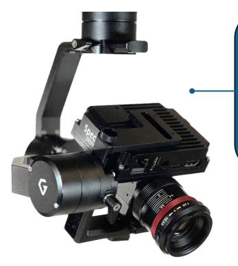
The MSDC is a multispectral drone camera for easy integration to drones with PixHawk flight controllers enabling capture of geotagged aerial images for further analysis in data mapping software.
