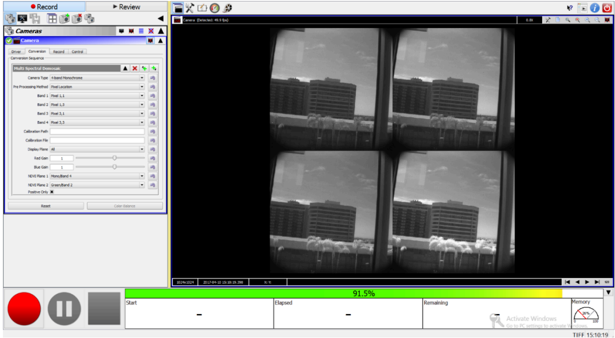
Figure 10.3. Real-time display of multispectral images in montage format. Example here collected with a 4-band multispectral camera for agriculture.
