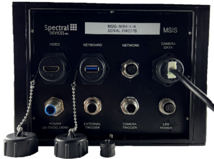
Figure 10.1. Control Box photos
