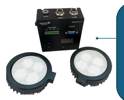
The MSLED-RGBN-2-4 consists of two LED modules each equipped with four independent LED channels - the conventional red, green, blue, as well as near-infrared channel. The dual LED illuminator creates a uniform diffuse lighting for a variety of multispectral imaging applications.
