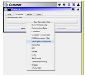
Figure 10.2. Multispectral conversion filters
