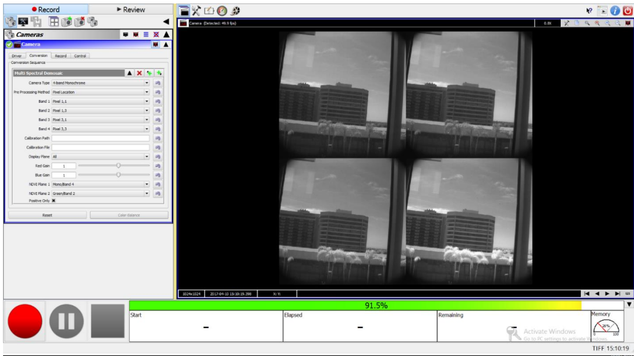
Figure 9.3. Real-time display of multispectral images in montage format. Example here collected with 4-band multispectral camera for agriculture.
