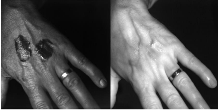
UV (left) and NIR (right) images of human hand with sun screen applied
