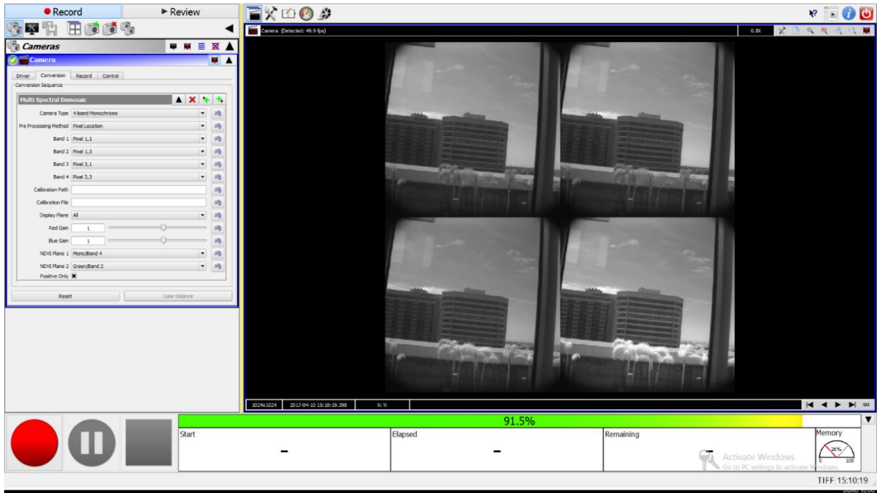
Figure 10.3. Real-time display of multispectral images in montage format. Example here collected with 4-band multispectral camera for agriculture.
