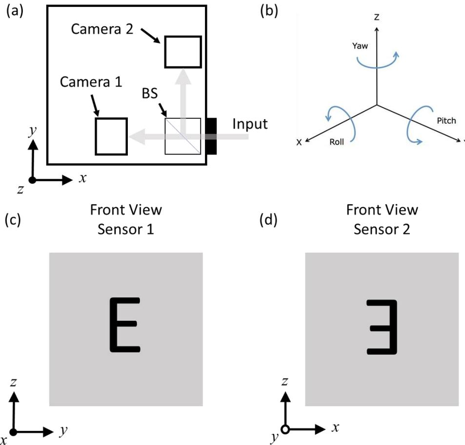
(a) General layout of cameras within the MSMC-2-2 showing orientation of cameras with respect to the beam splitter (BS) and the MSMC-2-2 coordinate system.
